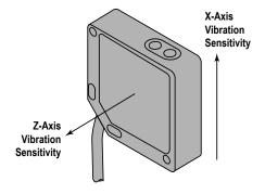
After determining the sensor direction and location, mount the sensor for the best possible vibration sensing accuracy. Mounting options in order from least effective to most effective are as follows:
