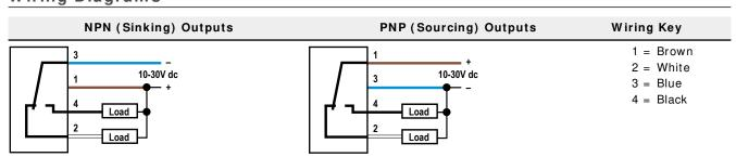
Cabled wiring diagrams are shown. Quick disconnect (QD) wiring diagrams are functionally identical.
