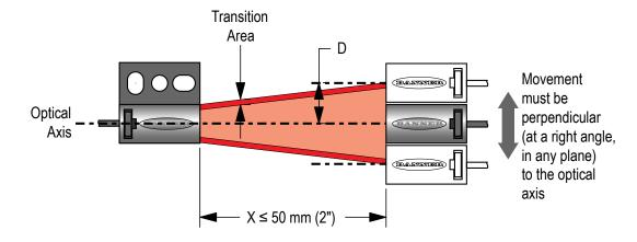
Model SFI-S1L is shown. The principle is the same for the other models. The optical beam pattern shown is exaggerated for clarity.
