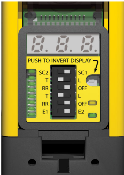
Figure 26. EZ-SCREEN Configuration DIP Switches (Receiver)
